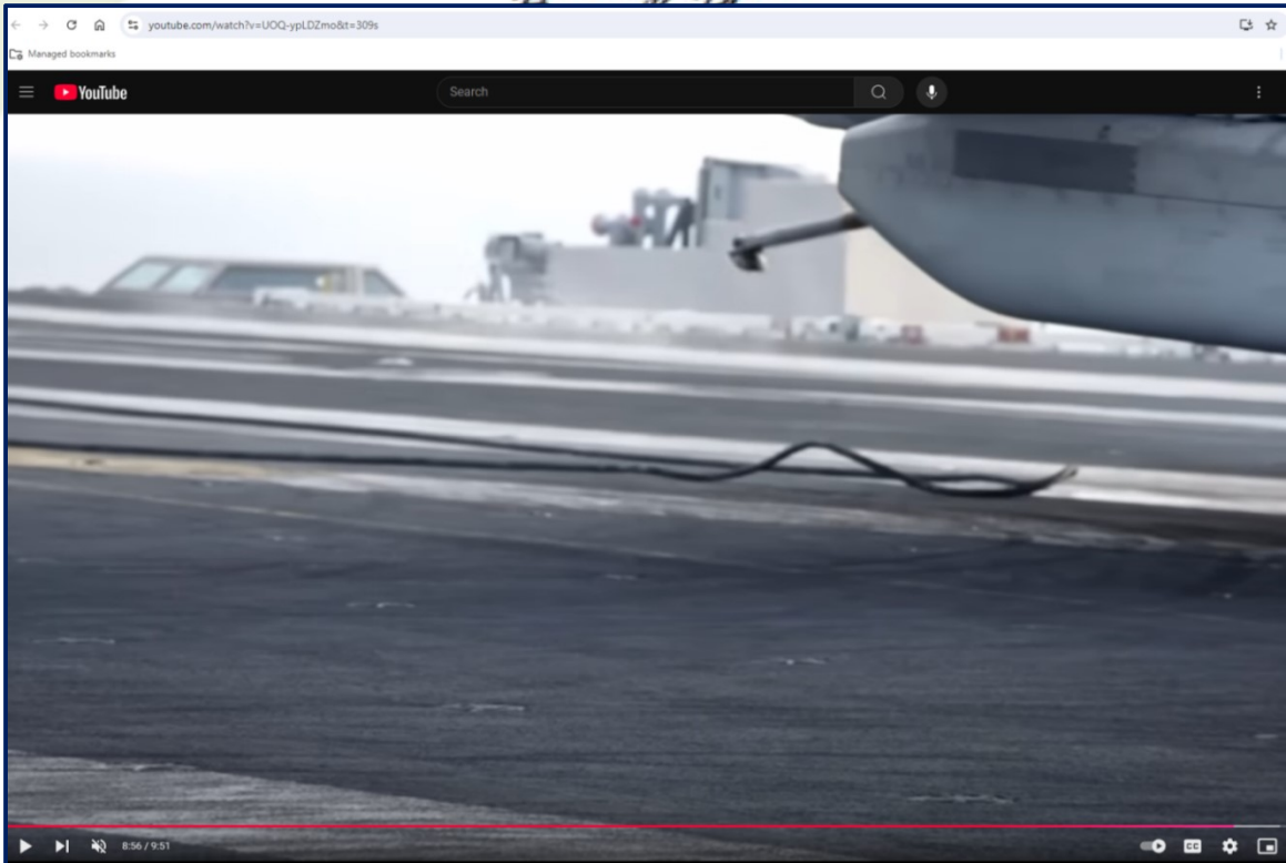
Figure-I2: Aircraft missed catching rope/cable
